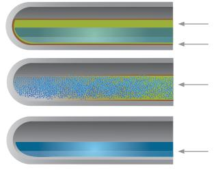
Bacteria forms inside irrigation lines due to organics (fertilisers, recycled water) in the water.
